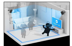
Top: Constellation through an IR-enabled camera (image credit: ifixit.com ) Bottom: HTC Vive room setup showing two base stations (image credit: HTC)
