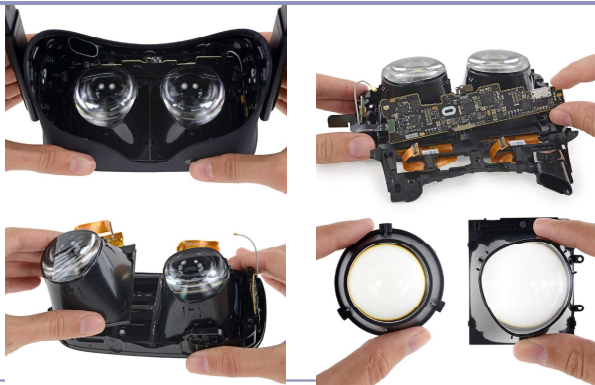
Teardown of an Oculus Rift CV1 showing details of lenses and displays https://www.ifixit.com/Teardown/Oculus+Rift+CV1+Teardown/90612
